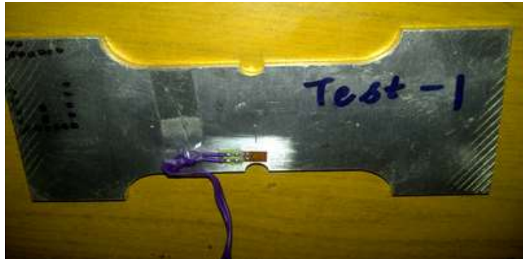
Fig. 6 (b) Positioning of strain gauge
