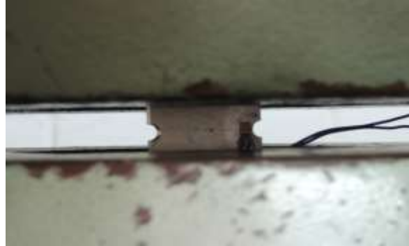
Fig. 8 Specimen fixed on UTM
