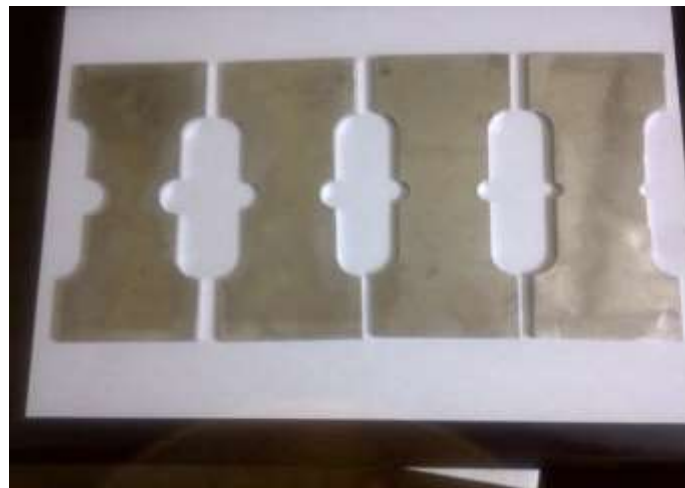
Fig. 4 Below shows the specimens fabricated by the wire cutting method.
